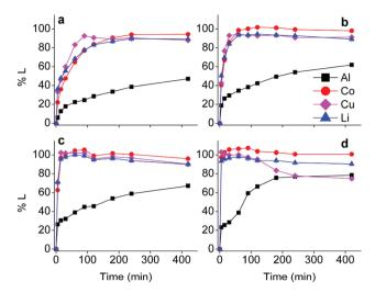
Fig. 1 Leaching efficiencies (%L) of LiCoO $_2$  + Al + Cu mixtures in choline chloride–citric acid DES as a function of time at different temperatures. Temperatures: room temperature (left above, a), 40 °C (right above, b), 60 °C (left below, c) and 80 °C (right below, d). DES: ChCl : CA 2:1+35 wt%  $H_2O$ . Leaching parameters: S:L=20 g  $L^{-1}$ , Al : LiCoO $_2=12$  wt%, Cu : LiCoO $_2=24$  wt% at 900 rpm.
