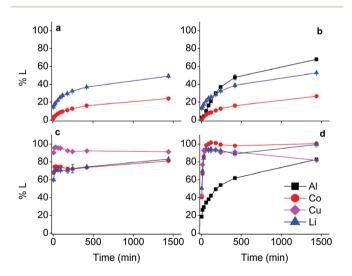
Fig. 3 Comparison of the effects of current collector metals on the leaching of lithium cobalt oxide by choline chloride–citric acid DES. Conditions: Only LiCoO<sub>2</sub> (left above, a), LiCoO<sub>2</sub> with Al (right above, b), LiCoO<sub>2</sub> with Cu (left below, c), LiCoO<sub>2</sub> with Al + Cu (right below, d). DES: ChCl : CA 2 : 1 +35 wt%  $H_2O$ . Leaching parameters: S: L=20 g  $L^{-1}$ , 40 °C, Al : LiCoO<sub>2</sub> = 12 wt%,  $Cu: LiCoO_2=24$  wt% at 900 rpm.
