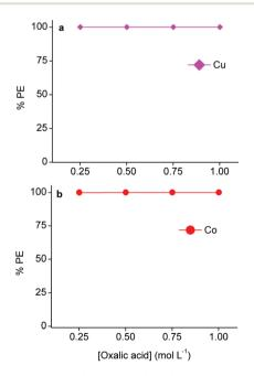
Fig. 9 Efficiencies of stripping precipitation of metal oxalates at different oxalic acid concentrations. (a) Cu(1/11) oxalate formation by stripping from loaded 60 vol% LIX 984 in an aliphatic diluent and (b) cobalt(II) oxalate formation by stripping from loaded undiluted waterpresaturated A336. The loaded LIX 894 and A336 contained 4.7 g  $L^{-1}$ Cu(I/II) and 9.8 g L<sup>-1</sup> Co(II). Phase ratio = 1:1, equilibration = 30 min, shaking speed = 2250 rpm, room temperature.
