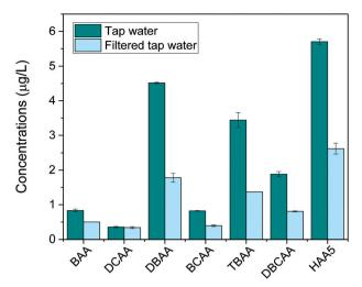
Fig. 5 Average concentrations (n = 2) of HAAs in tap water and after filtration with a household water pitcher filtration unit (Jata Hogar, model RF123x4)
