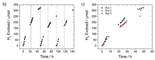
Fig. 6 (a) Images of free-standing film suspended in 5 vol% TEA before and after photocatalytic experiment; (b) hydrogen evolution of free-standing film of **FS-TEG** from a 5 yol% TEA mixture under  $\lambda > 420$  nm irradiation over a period of 141 hours with intermittent degassing (black dashed lines) and replacement of scavenger mixture (red dashed lines) (300 W Xe light source); (c) direct comparison of hydrogen evolution runs after replacing the scavenger mixture.
