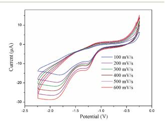
Fig. 5 Cyclic voltammogram of complex  $4^{tBu}$  at different scan rates versus Fc/Fc<sup>+</sup> measured in THF with 0.1 M [ $^n$ Bu<sub>4</sub>N][PF<sub>6</sub>].
