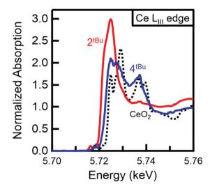
Fig. 6 Normalised HERFD-XAS spectra at the Ce  $L_{\rm III}$  absorption edge. The increased edge energy and doublet peak for  $4^{\rm fBu}$  (blue) compared with  $2^{\rm fBu}$ -Ce (red) confirm the Ce(iv) oxidation state of  $4^{\rm fBu}$ . The doublet peaks of  $4^{\rm fBu}$  also match those observed for CeO<sub>2</sub> (black, dotted), which serves as a Ce(iv) fingerprinting standard. Peak splitting in the CeO<sub>2</sub> HERFD spectrum has been attributed to 5d state splitting.  $^{43}$
