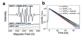
Fig. 3 (a) EPR spectra of DMPO-O2 adducts with cPMMA-BTPh2 as the photocatalyst in darkness and under blue light irradiation ( $\lambda$  = 460 nm, 1.2 W cm<sup>-2</sup>). (b) Time-resolved photoluminescence spectra of BTPh2 under N2 (black), under O2 (red), and with trans-anethole under N<sub>2</sub> (green) and in air (blue) with 20 mg mL<sup>-1</sup> of BTPh<sub>2</sub> and 2 mM trans-anethole in acetonitrile.
