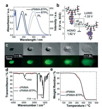
Fig. 1 (a) Comparison of the photoluminescence and UV/vis spectra of BTPh2 units and the polymer cPMMA-BTPh2 in the solid state and (b) DFT/B3LYP 6-31G(d) calculated electronic structures for the HOMO and LUMO of a simplified cPMMA-BTPh2. Potentials resulting from the CV measurements on cPMMA-BTPh<sub>2</sub>. (c) Optical microscopy images of cPMMA-BTPh2, swelling after exposure to CH3NO2. (d) FTIR and (e) TGA spectra of cPMMA-BTPh2 and the blank cPMMA sample.
