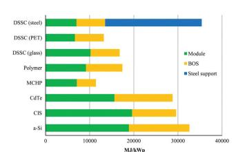
**Fig. 3** Cumulative energy demand for the production of a virtual 3 kW h solar harvesting rooftop photovoltaic installation for various thin-film technologies. Reproduced with permission from Elsevier.<sup>7</sup>
