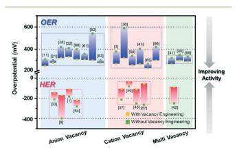
Fig. 8 Trend of the performance of recent vacancy-engineered electrocatalysts.
