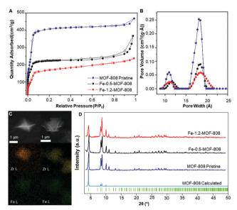
Fig. 1 (A) N<sub>2</sub> adsorption/desorption isotherms at 77 K showing the decrease in surface area upon iron incorporation. (B) Pore size distribution (PSD) data for pristine and Fe-SIM MOF-808 materials. (C) Mapping of Zr (yellow) and Fe (green) for Fe-0.5-MOF-808 (right) and Fe-1.2-MOF-808 (left). (D) PXRD data of the synthesized materials and their comparison with the calculated data for MOF-808, 19 including Bragg positions.
