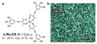
Fig. 2 (a) Molecular structure and phase behavior of the  $\Delta$  isomer of **Ru-C8**. (b) Polarized optical micrographs of the textures displayed by  $\Delta$ -**Ru-C8** in a Col<sub>n</sub> phase at 40 °C (after annealing).
