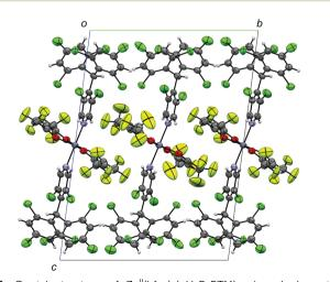
**Fig. 2** Crystal structure of  $Zn^{II}(hfac)_2(\alpha H-PyBTM)_2$  viewed along the a-axis. Disorders of the trifluoromethyl groups and central carbon atoms of  $\alpha H-PyBTM$  are omitted for clarity.
