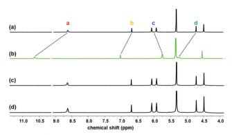
Fig. 1 Partial <sup>1</sup>H NMR spectra of (a) 1 (2 mM) and 1 with (b) excess LiCl(s), (c) excess NaCl(s), and (d) excess KCl(s) recorded in 10% CD<sub>3</sub>OD/CD<sub>2</sub>Cl<sub>2</sub>.
