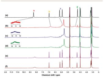
Fig. 3 <sup>1</sup>H NMR spectra of (a) **1** (5 mM) and **1** after extraction with (b) LiCl(aq), (c) LiCl(s), (d) a mixture of LiCl(s), NaCl(s) and KCl(s), (e) excess NaCl(s), and (f) excess KCl(s)
