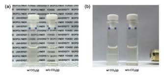
Fig. 4 (a) Turbidity and (b) the Tyndall effect of a solution containing the 1-LiCl complex after CO<sub>2</sub>(g) bubbling with deionized water.
