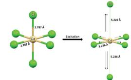
Fig. 2 (a) Absorption, excitation ( $\lambda_{em} = 385$  nm), and emission ( $\lambda_{exc} =$ 290 nm) spectra of (TDMP)CdCl<sub>4</sub>. (b) PL excitation vs. emission mapping of (TDMP)CdCl<sub>4</sub>, and (c) calculated distortion of  $[CdX_6]^{4-}$  motifs under excitation.
