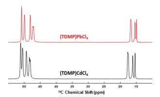
Fig. 3 <sup>1</sup>H-<sup>13</sup>C CP-MAS NMR spectra of (TDMP)CdCl<sub>4</sub> and (TDMP)PbCl<sub>4</sub>.
