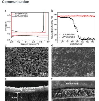
Fig. 1 Li metal performance in the selected electrolytes at room temperature. (a) Li plating/stripping curves and (b) long-term cycling performance of Li||Cu cells in LiFSI MP/FEC, and LiPF $_6$  EC/DEC at 0.5 mA cm $^{-2}$ ; top (c and d) and cross-section (e and f) views of the SEM images of Li deposits obtained in LiPF $_6$  EC/DEC (c and e) and LiFSI MP/FEC (d and f) at 1 mA h cm $^{-2}$  and 0.5 mA cm $^{-2}$ .
