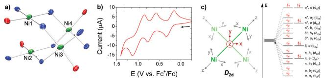
Fig. 1 (a) Partial solid-state structure of [Ni4] highlighting the inner core (see Fig. S15 for full structure, ESI†). (b) CV of [Ni4] in TCE (1 mM of [Ni4], 0.1 M [Bu<sub>4</sub>N][PF<sub>6</sub>] supporting electrolyte), glassy carbon working electrode, Pt wire counter electrode, and Ag wire pseudo-reference electrode. (c) Partial d-orbital splitting diagram for a  $D_{2d}$  tetrametallic core, ignoring ligand  $\pi$  interactions.
