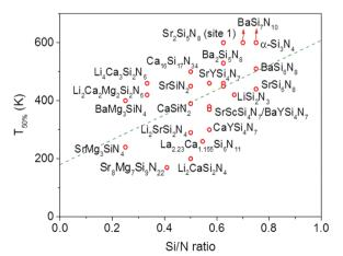
Fig. 4 Temperature at which 50% of the  $Eu^{2+}$  5d-4f emission is quenched ( $T_{50\%}$ ) versus the Si/N ratio of the Eu<sup>2+</sup> doped nitridosilicates. The dashed green lines is a linear fit through the data points to indicate the
