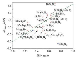
Fig. 7  $\Delta E_{\rm 5d-CB}$  versus the Si/N ratio in the Eu<sup>2+</sup> doped nitridosilicates. The straight line is a linear fit through the red data points. The blue squared data points represent exceptions discussed in the text.
