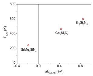
Fig. 5 Temperature at which 50% of the Eu<sup>2+</sup> 5d-4f emission is quenched  $(T_{50\%})$  versus the energy difference ( $\Delta E_{\rm 5d-CB}$ ) between the bottom of the host lattice conduction band and the lowest relaxed Eu<sup>2+</sup> 5d state for SrMg<sub>3</sub>SiN<sub>4</sub>:Eu<sup>2+</sup>, Ca<sub>2</sub>Si<sub>5</sub>N<sub>8</sub>:Eu<sup>2+</sup> and Sr<sub>2</sub>Si<sub>5</sub>N<sub>8</sub>:Eu<sup>2+</sup>.
