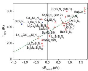
Fig. 6 Temperature at which 50% of the Eu<sup>2+</sup> 5d-4f emission is quenched ( $T_{50\%}$ ), versus the energy difference ( $\Delta E_{5d-CB}$ ) between the bottom of the host lattice conduction band and the lowest Eu<sup>2+</sup> 5d state. The straight green line is a linear fit through the red data points. The blue squared data points represent exceptions discussed in the text.
