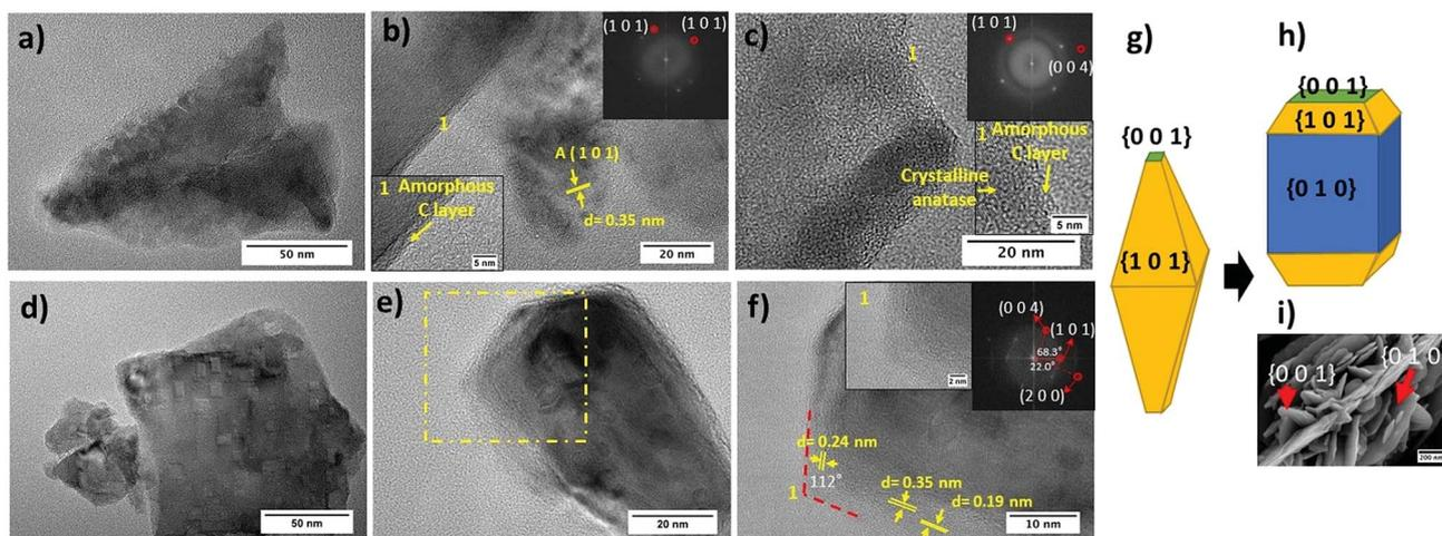
Fig. 4 TEM and HRTEM micrographs of (a–c)  $\text{TiO}_2$ -Rose-AD and (d–f)  $\text{TiO}_2$ -Rose-800. Fast Fourier transformation (FFT) patterns and inverse FFT image are shown in the inset of (b and c) and (f). (f) Region highlighted in (e). (g) Wulff construction of anatase crystals and (h) evolved shape with high exposure of  $\{0\ 1\ 0\}$  facets. (i) SEM micrograph highlighting the facets.
