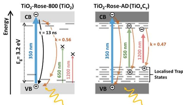
Fig. 9 Schematic diagram representing the difference in the photo-generated charge carrier dynamics for TiO<sub>2</sub>-Rose-800 and TiO<sub>2</sub>-Rose-AD when excited with 350, 650 or 1200 nm laser pulses with a photon flux of  $3.97 \times 10^{13}$ ,  $2.01 \times 10^{14}$  and  $1.22 \times 10^{14}$  photons cm<sup>-2</sup> pulse<sup>-1</sup>, respectively.
