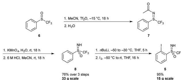
Scheme 1 Synthesis of iodosulfoximine compound **5**.  $\text{Tf}_2\text{O}$  = trifluoromethanesulfonic anhydride.
