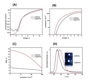
Fig. 9 (A) Current density-voltage characteristics (B) luminance vs. voltage. (C) EQE vs. luminance (D) normalized EL spectra of CzPhTrz and CzpPhTrz.
