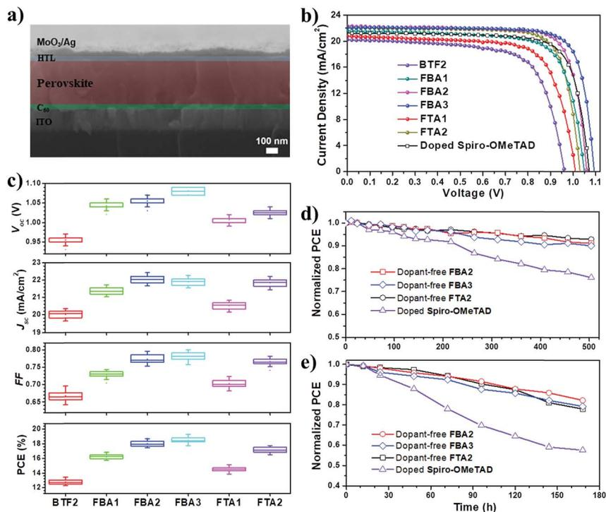
Fig. 6 (a) Cross-sectional SEM image of the complete PVSC device. (b)  $J$ - $V$  curves of the champion PVSCs with different dopant-free HTMs and doped spiro-OMeTAD. (c) Histograms of photovoltaic parameters. Environmental stability of PVSCs based on dopant-free FBA2, FBA3 and FTA2 and doped spiro-OMeTAD tested under simulated sunlight under nitrogen (d) or in ambient air with a humidity of 20–30% (e).
