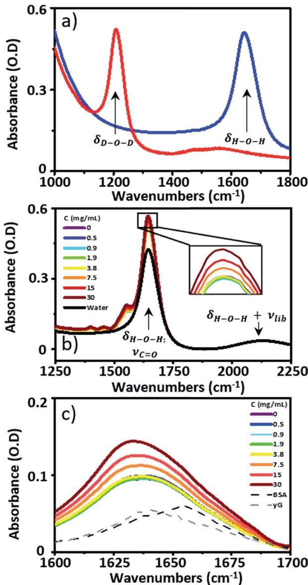
Fig. 1 (a) The IR absorption spectra of  $D_2O$  (red) and  $H_2O$  (blue). (b) IR absorption spectra of serum samples spiked with  $\gamma$ -globulins, pure  $H_2O$  is shown in black. The inset shows an expansion of the tip of the peak due to the  $H-O-H$  bending mode of water and the protein amide I band at  $1650\text{ cm}^{-1}$ . (c) IR absorption spectra of serum spiked with  $\gamma$ -globulins from (b) following subtraction of the  $H_2O$  spectrum.
