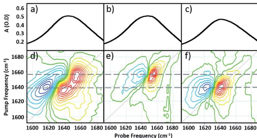
Fig. 3 IR absorption spectra of (a) serum (b) serum albumin (c)  $\gamma$ -globulins. 2D-IR spectra of (d) serum (e) serum albumin (f)  $\gamma$ -globulins. Dashed grey horizontal lines show peak positions of albumin and  $\gamma$ -globulins. The color scale is as shown in Fig. 2.
