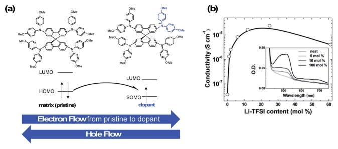
Fig. 3 (a) Integer charge-transport mechanism with molecular p-type dopant. Adapted with permission from ref. 95. Copyright 2007 American Chemical Society. (b) Effective spiro-OMeTAD conductivity and UV-Vis absorption spectra (inset) as function of the Li-TFSI content. These films were left for 78 hours in air before measurement. The solid-line is simply to aid the eye. Reproduced from ref. 96 with permission from the PCCP Owner Societies.
