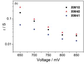
Fig. 7 Plots of (a)  $C_{\mu}$  and (b)  $\tau$  versus bias voltages of DSSCs based on XW10, XW40, and XW41.
