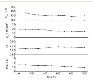
Fig. 8 Variation of the photovoltaic parameters ( $V_{\rm oc}$ ,  $J_{\rm sc}$ , FF, and PCE) with aging time for the DSSC device based on XW40/CDCA + Z1 measured under AM 1.5 illumination (100 mW cm $^{-2}$ ) at 60 °C over 1000 h.
