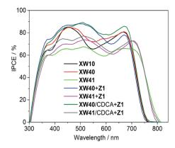
Fig. 6 IPCE action spectra for the DSSCs based on XW10,<sup>33</sup> Z1, XW40 and XW41.
