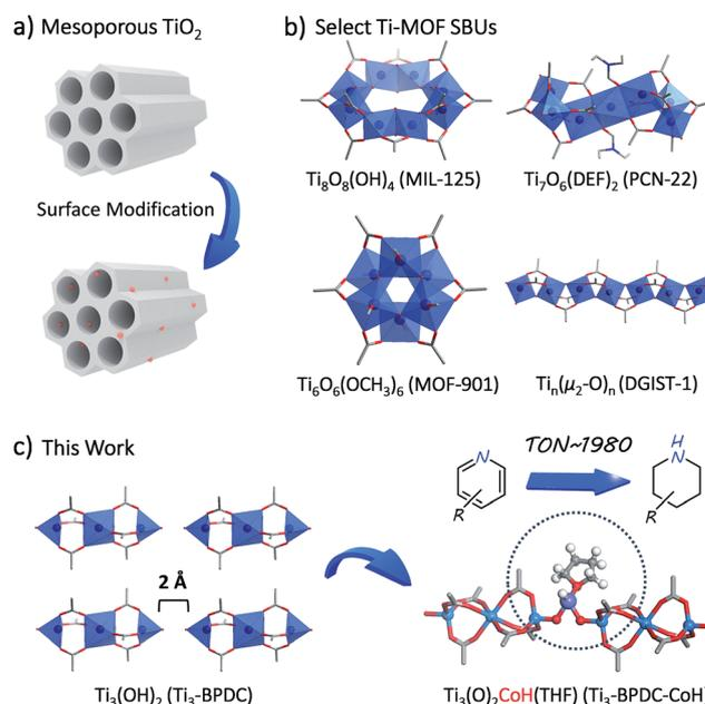
Fig. 1 (a) Surface modification of mesoporous TiO<sub>2</sub> generates functional materials. (b) Select Ti-MOF SBU structures (MIL-125, PCN-22, MOF-901, and DGIST-1). (c) Schematic illustration of novel Ti<sub>3</sub>(OH)<sub>2</sub> SBUs in Ti<sub>3</sub>–BPDC and their metalation to generate anchored Co<sup>II</sup>-H species for cascade reduction of N-heteroarenes.
