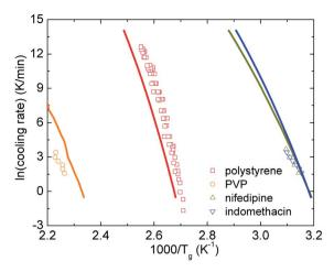
Fig. 6 The logarithm of cooling rate as a function of inverse glass transition temperatures of various amorphous drugs and polymers. Points are experimental data and solid curves correspond to our theoretical calculations using eqn (16).
