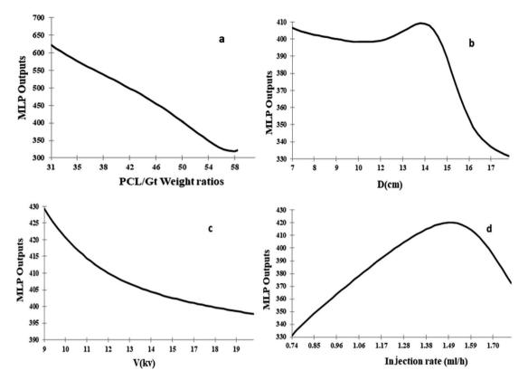
Fig. 10 The trend of the DPNFM<sub>MLP</sub> output changes upon varying: the (a) PCL/Gt weight ratio; (b) distance; (c) voltage; and (d) injection rate.
