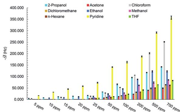
Fig. 8 Sensor responses to different VOCs concentration.
