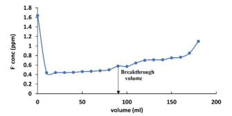
Fig. 7 Breakthrough curve for fluoride adsorption on to HAP-MMT.
