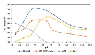
Fig. 4 The effect of pH on adsorption capacity of  ${\sf F}^-$  and adsorption percentage.
