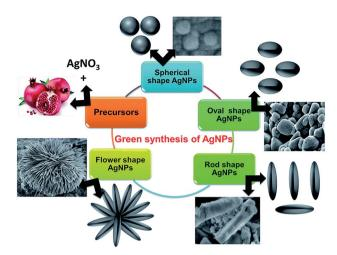
**Scheme 3** Graphical representation of synthesis of shape-specific silver nanoparticles using the green synthesis approach<sup>40b</sup> (adapted with permission from Royal Society of Chemistry, 2015).
