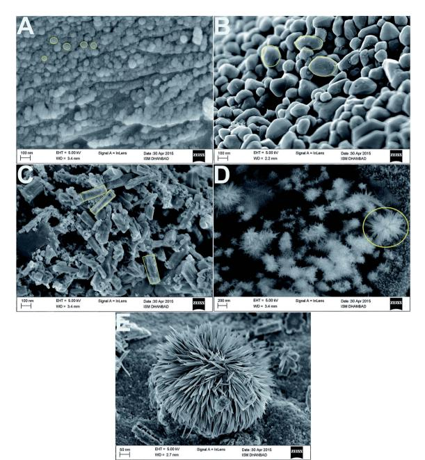
Fig. 12 FE-SEM images of the (A) spherical, (B) oval, (C) rod and (D) flower-shaped silver nanoparticles at low and (E) high magnifications<sup>40b</sup> (adapted with permission from Royal Society of Chemistry, 2015).
