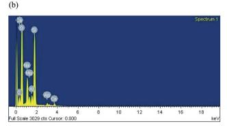
Fig. 3 (a) UV-Vis absorption spectra of the coating with different numbers of loading/reduction cycles; (b) EDX image of the coating with 4 dip/reduction cycles (PAA 20 mM)<sup>29</sup> (adapted with permission from SpringerNature, 2011).
