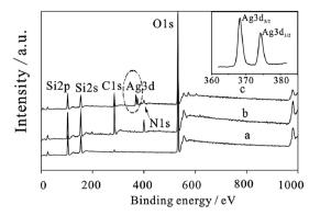
Fig. 14 XPS spectra of (a)  $mSiO_2$ , (b)  $mSiO_2@NH_2$  and (c)  $mSiO_2@-NH_2@Ag$ ; inset is the high resolution Ag 3d XPS spectra of  $mSiO_2@-NH_2@Ag^{41}$  (adapted with permission from Royal Society of Chemistry, 2015)
