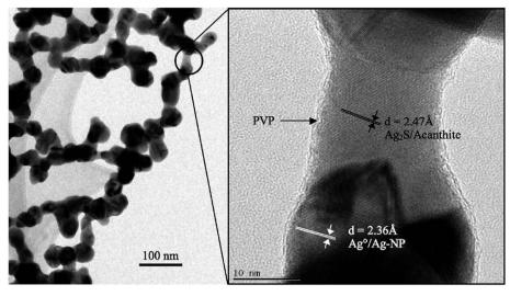
Fig. 6 TEM images of partly sulfidized Ag-NPs. The right image is at higher magnification and is centered on one of the nanobridges observed at low magnification (left image)<sup>34c</sup> (adapted with permission from American Chemical Society, 2012).
