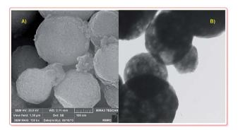
Fig. 1 FE-SEM (A) and TEM (B) analysis of Fe<sub>2</sub>O<sub>3</sub> hollow spheres.<sup>5</sup>
