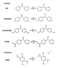
Scheme 1 Redox reactions of the analytes and catholyte.
