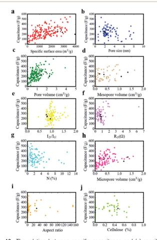
Fig. 10 The relation between specific capacitance and (a) specific surface area, (b) pore size, (c) pore volume, (d) mesopore volume, (e) the intensity ratio of ID/IG, (f)  $R_s$  (g) N-doping amount, (h) micropore volume, (i) aspect ratio, (j) cellulose amount.
