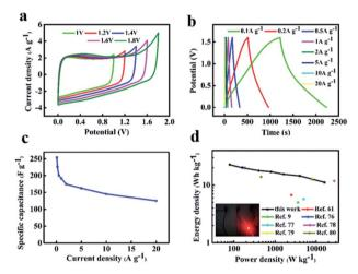
Fig. 9 Electrochemical measurements of the assembled NFAC-c// NFAC-c supercapacitor in 1 M Na<sub>2</sub>SO<sub>4</sub> electrolyte: (a) CV curves in various potential window at a scan rate of 50 mV  $s^{-1}$ . (b) GCD curves at different current densities. (c) Specific capacitances at different current densities. (d) Ragone plot. The inset is the lightened LED light.
