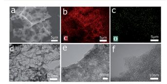
**Fig. 6** (a) SEM image of the obtained three-dimensional porous active carbon (NFAC-c). (b) Corresponding elemental mapping images of C atom and O atom in (c). (d) TEM image of NFAC-c. (e) and (f) HRTEM image of NFAC-c.
