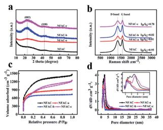
Fig. 7 (a) XRD profiles of NFAC-x. (b) Raman spectra of NFAC-x. (c) N<sub>2</sub> adsorption/desorption isotherm of NFAC-x. (d) Pore size distributions of NFAC-x. The inset shows magnified section of pore diameter ranging from 1 nm to 5 nm.
