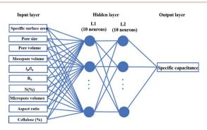
Fig. 2 Artificial neural network model for supercapacitor.
