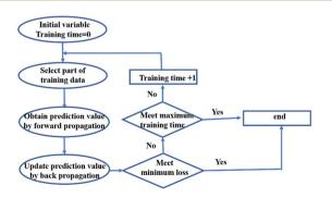
Fig. 3 The program illustration of back propagation algorithm.
