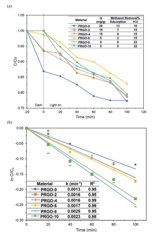
Fig. 9 (a) Adsorption and PCO of methanol and (b) pseudo-first order kinetics of methanol PCO by PRGOs.
