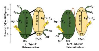
Fig. 11 Schematic diagram of electron transfer in the ZnO@Sn $_3$ O $_4$ .
