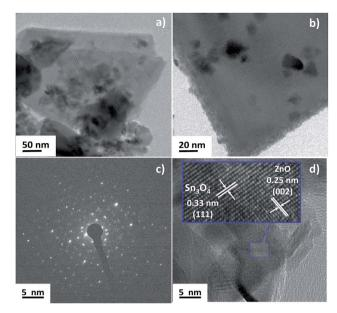
Fig. 4 TEM (a and b), SAED pattern (c), HRTEM (d) images of  $ZnO@Sn_3O_4$ , respectively.
