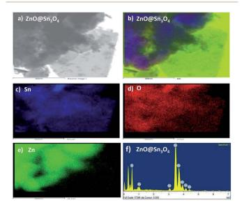
Fig. 5 (a) TEM image of  $ZnO@Sn_3O_4$  for EDS; (b-f) EDS element mapping data of Zn, Sn and O elements for  $ZnO@Sn_3O_4$ , respectively.
