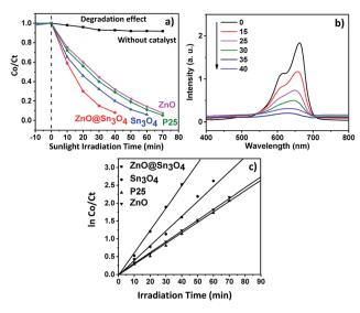
Fig. 9 (a) Plot of change in absorbance vs. irradiation time in the presence of ZnO, Sn<sub>3</sub>O<sub>4</sub>, P25 and ZnO@Sn<sub>3</sub>O<sub>4</sub>; (b) spectral changes of degradation of MB dye in the presence of ZnO@Sn<sub>3</sub>O<sub>4</sub>; (c) pseudofirst-order kinetic plots of  $ln(C_0/C_t)$  vs. irradiation time for the degradation of methylene blue (MB) using ZnO, Sn<sub>3</sub>O<sub>4</sub>, P25 and ZnO@Sn<sub>3</sub>O<sub>4</sub>.
