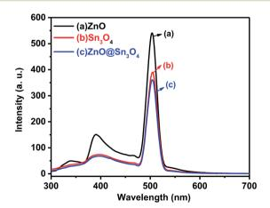
Fig. 7 PL spectra of (a) ZnO, (b) Sn<sub>3</sub>O<sub>4</sub> and (c) ZnO@Sn<sub>3</sub>O<sub>4</sub>.
