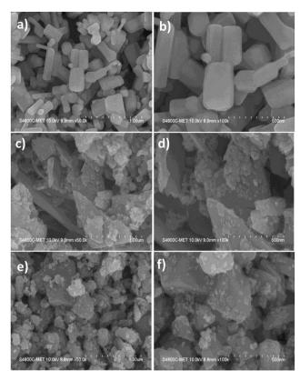
Fig. 3 FESEM images of (a and b) ZnO, (c and d)  $Sn_3O_4$ , (e and f) ZnO@ $Sn_3O_4$ , respectively.
