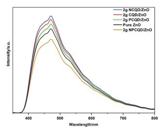
Fig. 11 PL spectra of the as-synthesized multi-shelled ZnO composites decorated with different element-doped carbon quantum dots.
