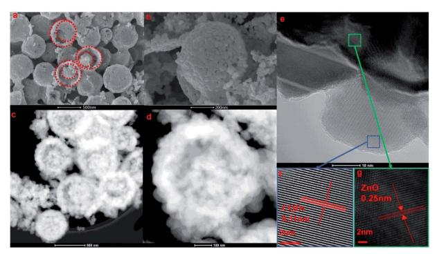
SEM images (a and b), scanning TEM images (c and d), and HRTEM images (e-g) of the prepared 2 g-NPCQD/ZnO composites.
