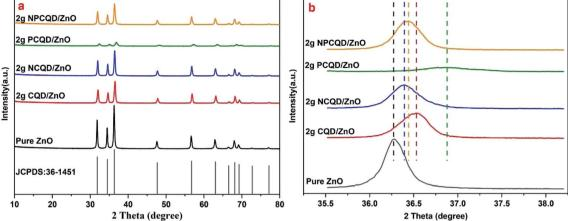
Fig. 2 XRD patterns of the CQD/ZnO composites.
