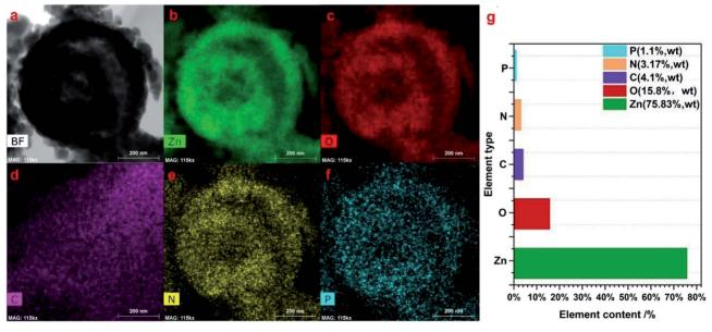
Fig. 5 The corresponding elemental mapping images (a-f) and the elemental distribution of the prepared 2 g-NPCQD/ZnO composites (g).
