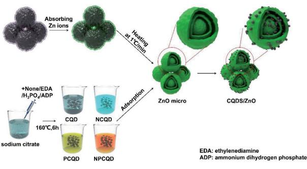
Fig. 1 Schematic of the formation process of the carbon quantum dot-decorated multi-shelled ZnO composites (CQD/ZnO).
