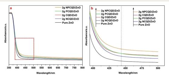
Fig. 9 UV-Vis absorption spectra (a) and band edges of the as-synthesized multi-shelled ZnO composites decorated with different element -doped carbon quantum dots (b).
