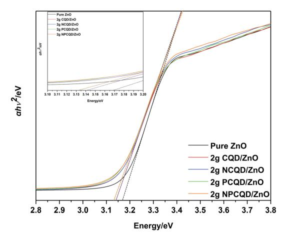
Tauc plot of the as-synthesized multi-shelled ZnO composites decorated with different element-doped carbon quantum dots.
