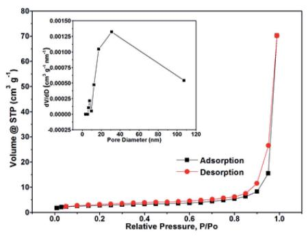
Fig. 3 N<sub>2</sub> adsorption-desorption isotherm and pore size distribution (inset) of NPCQD/ZnO.
