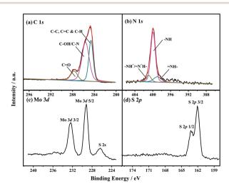
Fig. 1 High-resolution XPS spectra of (a) C 1s, (b) N 1s, (c) Mo 3d, and (d) S 2p of  $MoS_2$ -PANI/rGO nanocomposite.
