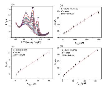
Fig. 6 (a) DPV curves of MoS<sub>2</sub>-PANI/rGO/GCE in 0.1 M PBS (pH 7.0, 0.1 M KCl) containing AA, DA, and UA with different concentrations. The concentration from bottom to top: 30  $\mu$ M to 3.0 mM for AA, 3.0 to 300  $\mu$ M for DA, and 2.0 to 200  $\mu$ M for UA, respectively. The plots of the oxidative peak currents *versus* the concentrations of (b) AA, (c) DA, and (d) UA.
