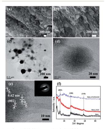
Fig. 2 (a and b) FE-SEM images of MoS<sub>2</sub>-PANI/rGO nanocomposite; (c) TEM and (d and e) HR-TEM images of 3D MoS<sub>2</sub>-PANI/rGO nanocomposite (the inset in (e) is the corresponding SAED pattern), and (f) XRD patterns of the MoS<sub>2</sub>, MoS<sub>2</sub>/rGO and MoS<sub>2</sub>-PANI/rGO samples.
