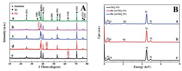
Fig. 2 (A) XRD patterns of: (a) 20 s Au/TiO<sub>2</sub> NTs; (b) 30 s Au/TiO<sub>2</sub> NTs; (c) 40 s Au/TiO<sub>2</sub> NTs; (d) 50 s Au/TiO<sub>2</sub> NTs; (e) 60 s Au/TiO<sub>2</sub> NTs. (B) EDS spectrum of: (a) TiO<sub>2</sub> NTs; (b) 40 s Au/TiO<sub>2</sub> NTs; (c) 50 s Au/TiO<sub>2</sub> NTs.
