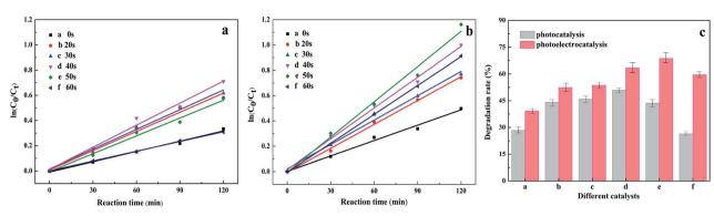
Fig. 6 (a) PC performances of the  $Au/TiO_2$  NTs for the degradation of nitrobenzene under the irradiation of UV light after 2 h; (b) PEC performances of the  $Au/TiO_2$  NTs for the degradation of nitrobenzene under the irradiation of UV light after 2 h; (c) degradation rate of nitrobenzene under different reaction systems after 2 h.
