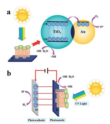
Scheme 2 (a) PC mechanism of the  $Au/TiO_2$  NTs; (b) PEC mechanism of the  $Au/TiO_2$  NTs.
