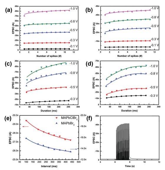
Fig. 4 SNDP of (a) MAPbClBr2- and (b) MAPbBr3-based artificial synapses at different voltages. The SDDP statistical graphs of (c) MAPbClBr2- and (d) MAPbBr<sub>3</sub>-based artificial synapses at different voltages. (e) SRDP statistical graphs (-0.5 V). (f) EPSCs triggered by 30 consecutive pulses (-0.5 V).
