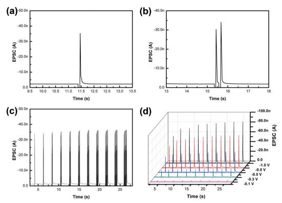
Fig. 3 (a) EPSC triggered by a single pre-synaptic spike (-0.5 V, 25 ms duration) in a MAPbClBr<sub>2</sub>-based artificial synapse. (b) EPSC triggered by a pair of pre-synaptic spikes with an interval time of 240 ms in a MAPbClBr<sub>2</sub>-based artificial synapse. (c) SNDP from 1 to 11 spikes (-0.5 V) in a MAPbClBr<sub>2</sub>-based artificial synapse. (d) SDDP at different pulse voltages in a MAPbClBr2-based artificial synapse.
