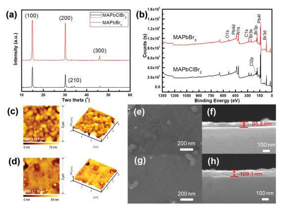
Fig. 2 (a) XRD patterns of the MAPbClBr<sub>2</sub> and MAPbBr<sub>3</sub> HP films. (b) XPS full scan spectra of the MAPbClBr<sub>2</sub> and MAPbBr<sub>3</sub> HP films. (c) AFM images of the MAPbClBr2 thin film. (d) AFM images of the MAPbBr3 thin film. Top-view SEM images of the (e) MAPbClBr2 and (g) MAPbBr3 thin films. Cross-sectional SEM images of the (f) MAPbClBr2 and (h) MAPbBr2 thin films.
