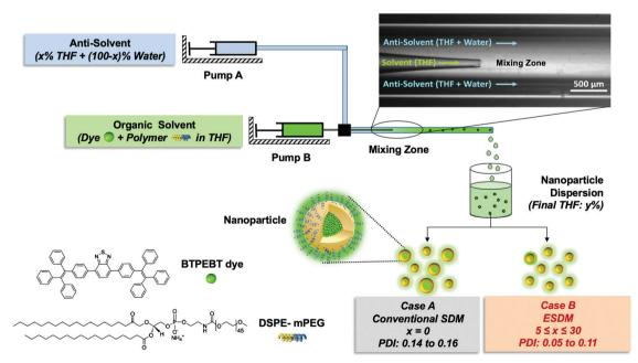
Fig. 1 Schematic of the microfluidic glass capillary mixer for the synthesis of monodisperse BTPEBT-loaded DSPE-mPEG<sub>2000</sub> NPs. Case A represents the synthesis of NPs through conventional SDM with 100% water (x = 0) from the outlet stream (pump A). Case B depicts the synthesis through ESDM with a mixture of THF (x%) and water (100 - x%) in the outlet stream for the preparation of highly monodisperse NPs (PDI values as low as 0.05).
