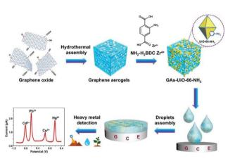
Fig. 7 Synthesis of the GAs-UiO-66-NH<sub>2</sub> composite via the in situ growth of the UiO-66-NH2 crystal on the GAs Matrix and the determination of heavy metal ions with the modified electrode. Reprinted from ref. 74 with permission from American Chemical Society.
