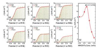
Fig. 5 Photocurrent density-potential curves of PEC devices based on colloidal heterostructured QD sensitized TiO2-MWCNTs hybrid photoanodes with different concentrations of MWCNTs under dark, continuous and chopped illumination (AM 1.5G, 100 mW cm<sup>-2</sup>): (a) 0.0 wt%; (b) 0.010 wt%; (c) 0.015 wt%; (d) 0.020 wt%; (e) 0.025 wt% and (f) 0.030 wt%. (g) Variation of current density at 1.0 V vs. RHE under 100 mW cm<sup>-2</sup> illumination with the concentration of MWCNTs.
