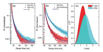
Fig. 4 Comparison of the transient PL curves of heterostructured QDs: (a) deposited onto a  $\rm ZrO_2$  and  $\rm TiO_2$  mesoporous film; (b) deposited onto a  $\rm ZrO_2$  mesoporous film and QDs with electrolyte. The excitation wavelength is  $\lambda_{\rm ex}=444$  nm. (c) Comparison of the spatial probability distribution value  $\rho(r)$  of the electron and hole as a function of QD radius r (nm) (H=2.15 nm, red for hole and cyan for an electron).
