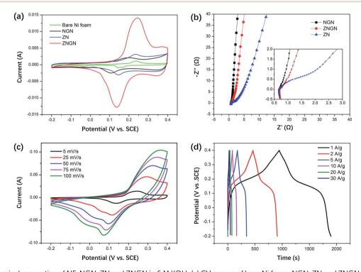
Fig. 7 Electrochemical properties of NF, NGN, ZN and ZNGN in 6 M KOH: (a) CV curves of bare Ni foam, NGN, ZN and ZNGN at  $100 \text{ mV s}^{-1}$  scan rate in the potential range from -0.2 to 0.4 V; (b) Nyquist plots of NGN, ZNGN and ZN; (c) CV curves of ZNGN at different scan rates ranging from 5 to 100 mV s; and (d) comparison of the galvanostatic charge/discharge curves at different current densities in the potential window from -0.2 to 0.4 V.
