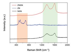
Fig. 3 Raman spectra of ZNGN, ZN, and NGN.
