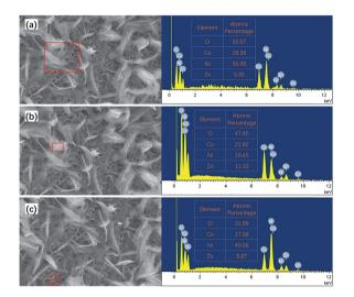
Fig. 5 EDS results of (a) dual-morphology  $ZnCo_2O_4$ , (b) feather-like  $ZnCo_2O_4$ , and (c)  $ZnCo_2O_4$  nanosheet .
