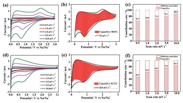
Fig. 7 CV curves of (a) N/S-HCNF (d) and N-HCNF electrodes at different scan rates. The capacitive contribution to the sodium ion storage marked by the shaded region at a scan rate of  $10.0 \text{ mV s}^{-1}$  of the as-synthesized (b) N/S-HCNFs and (e) N-HCNFs. Normalized contribution ratio of capacitive capacities at different scan rates of the as-synthesized (c) N/S-HCNFs and (f) N-HCNFs.
