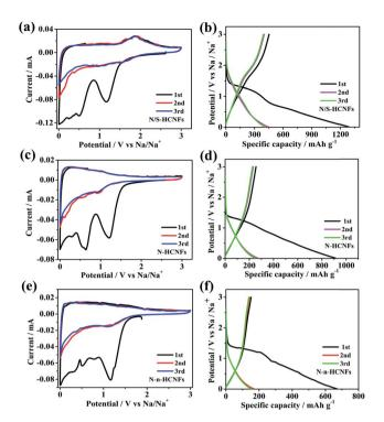
Fig. 5 CV curves of N/S-HCNFs (a), N-HCNFs (b) and N-n-HCNFs (c) at a scan rate of  $0.1\,\text{mV}\,\text{s}^{-1}$ ; the first three GCD profiles of N/S-HCNFs (d), N-HCNFs (e), and N-n-HCNFs (f) at  $0.05\,\text{A}\,\text{g}^{-1}$ .
