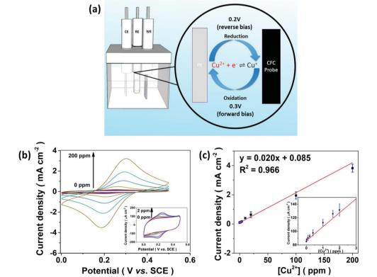
Fig. 4 (a) A diagram illustrating the E-chem processes on the CFC-UCNP probe. (b) CV curves of the CFC-UCNP probe in response to 0-200 ppm  $Cu^{2+}$  ions recorded within the potential window of 0-0.5 V at 100 mV s<sup>-1</sup>. (c) The linear relationship between the E-chem signals and  $[Cu^{2+}]$  obtained at 0.3 V. The insets are the enlarged plots for 0-2 ppm  $Cu^{2+}$  ions.
