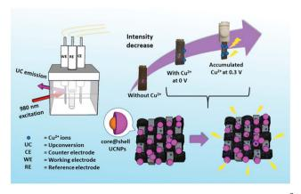
Fig. 1  $\,$  A schematic diagram showing the CFC-UCNP probe for  $\,$  Cu $^{2+}$  ion sensing under the E-chem assistance.
