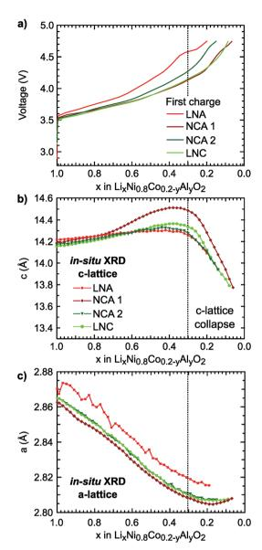
**Fig. 1** (a) First charge profile for layered oxide cathodes with chemical formula  $\text{LiNi}_{0.8}\text{Co}_{0.2-y}\text{Al}_y\text{O}_2$  ( $0 \le y \le 0.2$ ) to 4.75 V at 10 mA g<sup>-1</sup> (vs. Li metal) and at RT. *In situ* (b) c- and (c) a-lattice parameters for the first charge at C/50 to 4.75 V followed by a potentiostatic hold at 4.75 V for the Ni-rich systems. The c- and a-lattice parameters were calculated from the (003) peak and the (101) and (003) peaks, respectively.
