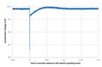
Fig. 4 A typical high-voltage spike in the acceleration voltage as recorded on the oscilloscope (see Fig. 1) due to flashovers. The horizontal axis covers a time interval of approximately 0.25 seconds. This time axis range therefore represents only a fraction (approximately a quarter) of a complete 1.049 second cycle exactly when a signal spike in the TE data plot also occurs, with an exactly matching timestamp. Each cycle is represented as a single symbol in Fig. 3.
