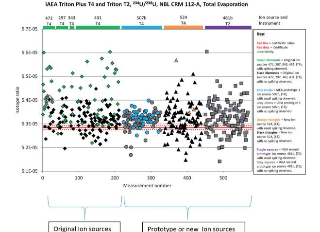
Fig. 9 QC chart displaying total evaporation  $^{234}$ U/ $^{238}$ U data collected on NBL 112-A certified reference material with various ion sources on the IAEA TIMS Triton Plus 'T4' and Triton 'T2'. Pink circled measurement discussed in Fig. 3.
