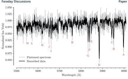
Fig. 1 Absorption spectrum in a range from 5500 Å to 6000 Å of  $C_{20}H_{10}^+$  complexed with a single He atom. The flattened raw spectrum is shown in gray and is overlaid with a spectrum where the data has been smoothed (moving average over 10 nearest neighbors) for easier viewing. All of the analysis is performed on the unsmoothed dataset. Identified absorption lines are labeled and their positions are reported in Table 1.
