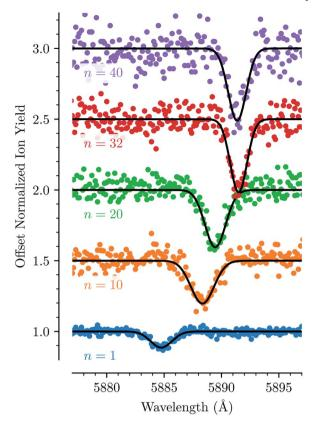
Fig. 2 The absorption feature of  $\mathrm{He}_n\mathrm{C}_{20}\mathrm{H}_{10}^+$  near 5885 Å (line D) shown for different numbers of n. The line is redshifted in a non-linear fashion up to n=32, after which the position is very slightly blue-shifted again. Gaussian fits are shown as solid black lines.
