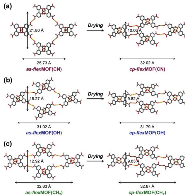
**Fig. 2** Comparison between the *as*-synthesised (*as*) and closed-pore (*cp*) phases of (a) *flexMOF(CN)*, (b) *flexMOF(OH)*, and (c) *flexMOF(CH<sub>2</sub>)* in rectangular dimension. The macrocycles and hydrogen atoms are omitted for clarity. Colour scheme: Ni, yellow; C, grey; O, red.
