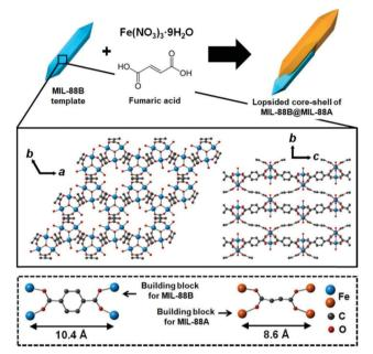
Scheme 1 Schematic representation of the preparation of the lopsided core-shell of MIL-88B@MIL-88A. Ball-and-stick representation for MIL-88B. MIL-88A has a similar 3D hexagonal structure and topology to the MIL-88B template; however, the cell parameters of MIL-88A are significantly different to those of MIL-88B, because a considerably short organic linker (fumaric acid) is involved in the growth of MIL-88A, compared with H2BDC required for MIL-88B.
