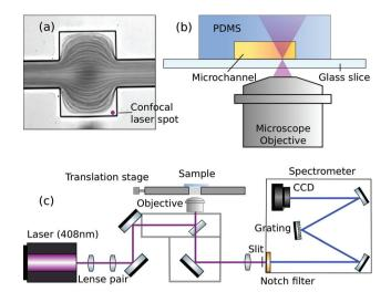
Fig. 2 Microfluidic Raman setup. (a) The localized cell-free plasma domain in microfluidic whole blood stream is probed by confocal Raman spectroscopy. (b) The Raman laser penetrates both the microfluidic channel and the PDMS host material (c) The microfluidic chip is mounted on the translation stage of an inverted microscope with confocal laser excitation at 408 nm. Raman emission is analyzed by an imaging dispersive spectrometer.
