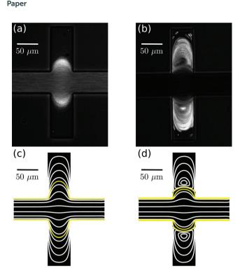
Fig. 4 Different flow patterns for the same in-plane channel geometry, but different channel depths of  $h=20~\mu m$  (a, c) and  $h=40~\mu m$  (b, d). Panels (a–b) show the standard deviation of microfluidic experiments whereas panels (c–d) illustrate the streamlines of corresponding creeping flow simulations.
