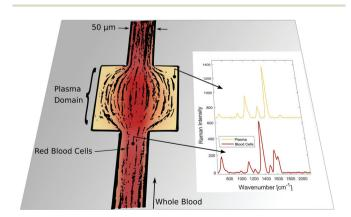
**Fig. 1** Instantaneous blood plasma fractionation appears adjacent to the channel walls of a geometric expansion in microfluidic whole blood flow. Local Raman spectroscopy on plasma domains (orange) is different compared to domains of streaming whole blood (red) where Raman scattering originates from cellular hemoglobin.<sup>4</sup> The Raman excitation wavelength is 408 nm.
