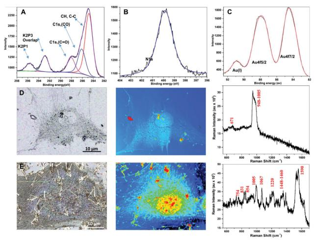
Fig. 3 High-resolution XPS spectra showing (A) carbon (C 1s), (B) nitrogen (N 1s), and (C) gold 4f7/4f5 nanoribbon-associated orbital binding energies of MCF7 cells in serum-free culture medium. Typical optical (D and G), SERS map images (E and H) and mean SERS spectrum (F and I) of twelve spectra at different points inside the MCF7 cell nucleus without (D-F) and with gold (G-I) nanoribbon synthesis.
